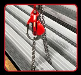
Often used with joists, trusses or to haul bulk of materials at site or load onto truck or ship
