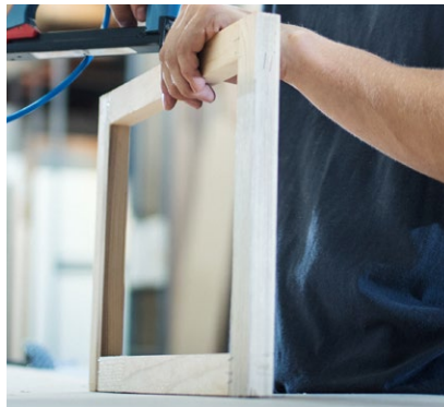
Butt-joint glued and stapled
