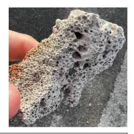
RAAC products were first introduced into the UK market in the 1950s and until the mid-1980s were increasingly used in the construction industry. Due to its lightweight, fire resistance and thermal performance, RAAC became popular for use in roof decks and was extensively used as such in both commercial buildings and, particularly, in public sector buildings such as schools, colleges and hospitals.
