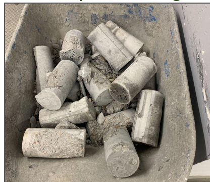
(From Left to Right) Figure 16: 6" by 12" Testing Molds, Figure 17: Concrete Samples After Compressive Strength Test
