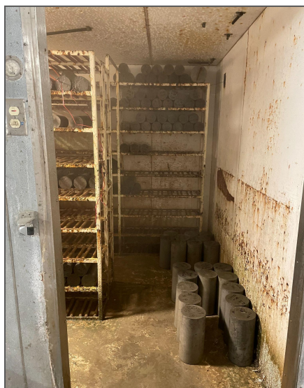
(From Left to Right) Figure 16: 6" by 12" Testing Molds, Figure 17: Concrete Samples After Compressive Strength Test
