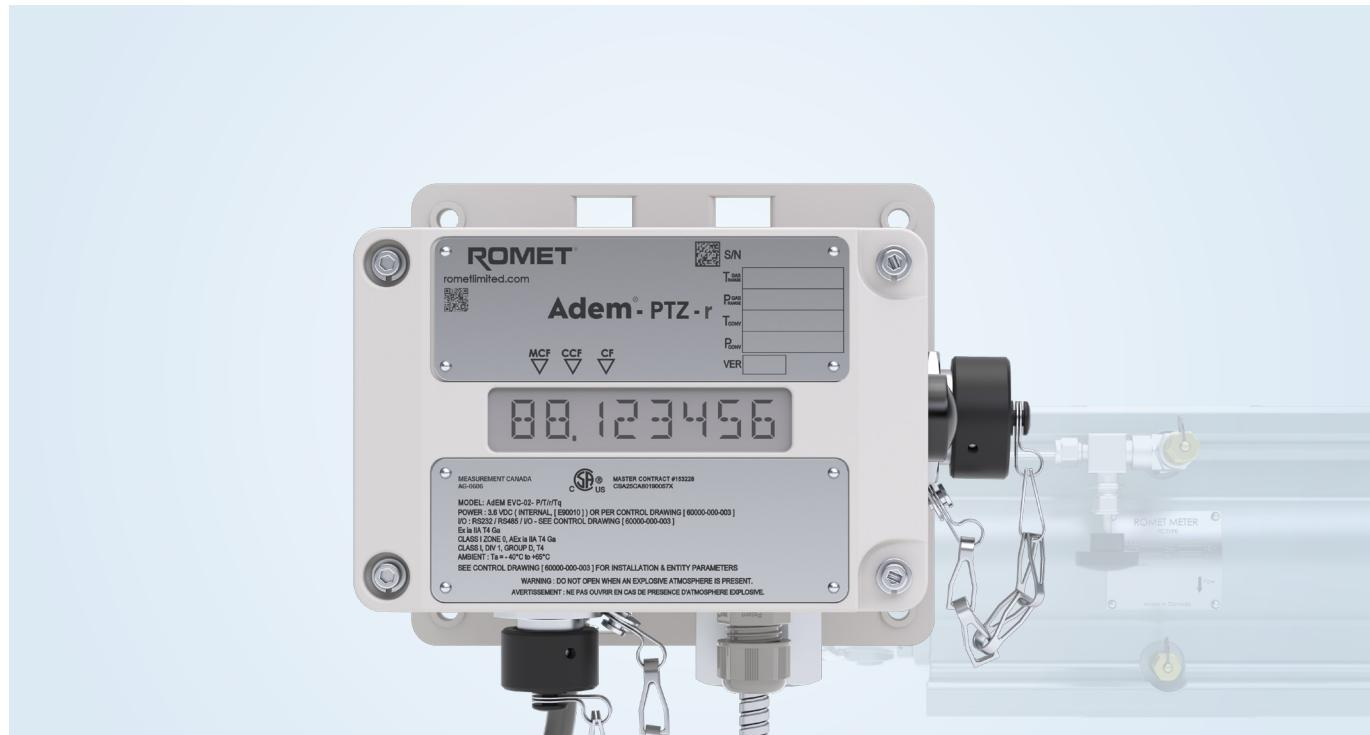
Romet's Adem®-PTZ-r is a remote mount electronic volume corrector module with the ability to account for temperature, pressure and supercompressibility. Compatible with any meter with a standard dry contact pulse output, the Adem®-PTZ-r has a compact, durable, service-free, tamperproof, and weather resistant design with a high level of accuracy and customization.
