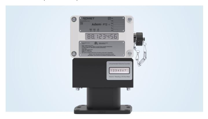
Romet's Adem®-PTZ-MI combines the data generation benefits and remote installation flexibility of Adem®-PTZ-r with the capability to collect data from instrument drive measurement devices. It is compatible with any meter equipped with standard CW or CCW Instrument Drive (ID or DCID) having suitable mounting platform, including ID rotary meters, large diaphragm meters, and turbine meters.
