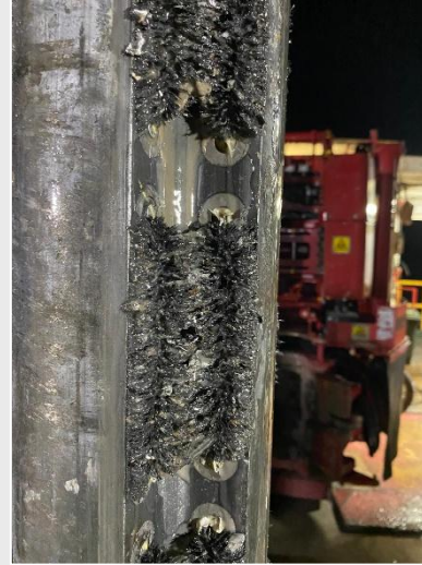
Metal buildup on string magnets
