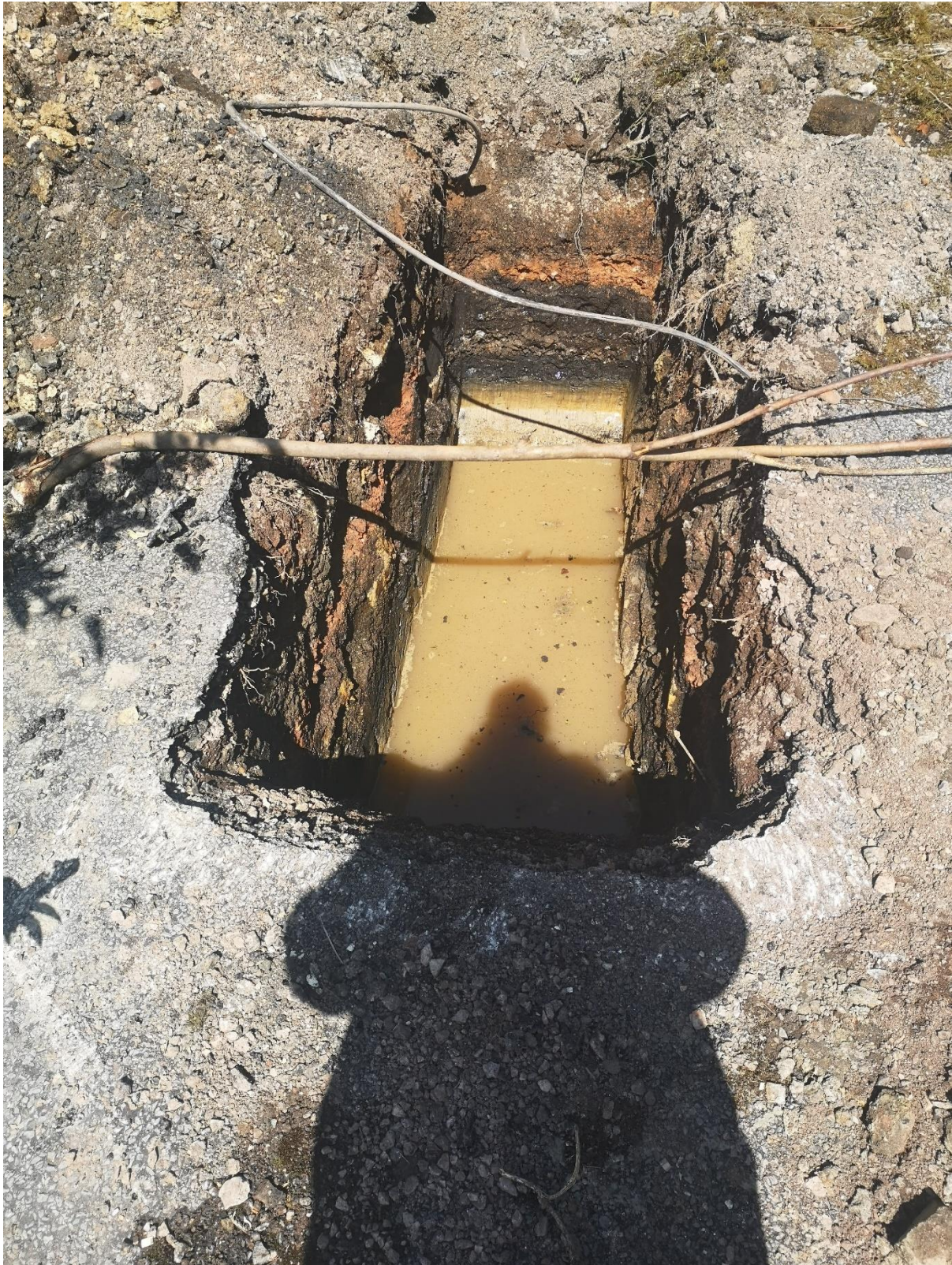
Figure 15 Engineer's test pit showing layers of material levelling up site in sections (Photo D. Bailey).
