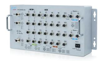
The EN50155 certified managed PoE switch ITP-12164XTM-12PH, that provides 4 10Gigabit, 16 Gigabit M12 X-code Ethernet ports and 12 Megabit M12 D-code, features total 12 ports PoE and supports a variety of PoE operation functions, including automatic detection of PoE device power, automatic reset, PoE scheduling, etc.
