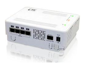
CTC Union Technologies unveils the next generation CPE switch, QSW-4204M, which supports multigigabit technology for active Ethernet based FTTH application. This new CPE switch is designed with 1 ports 10M/100M/1Gbps RJ45 and 4 ports 10M/100M/1G/2.5Gbps as well as 2 ports 1G/10Gbps SFP+ based fiber optics. As usual, the QSW-4204M adopts the evolutionary cable tray structural design to help the installer more easily and protectively manage the excess fiber within the unit.
