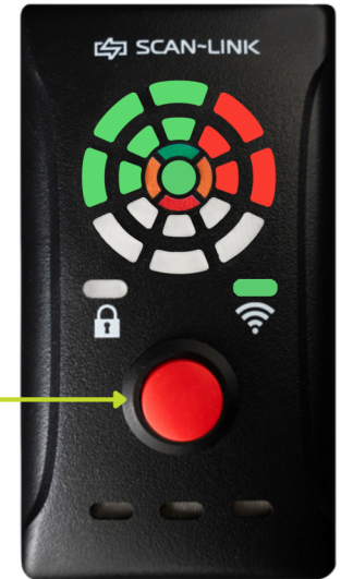
Figure 1: 3.0 Display Unit at maximum volume
