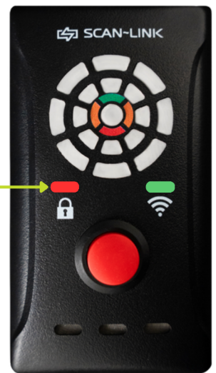
Figure 2: 3.0 Display Unit with Operator Lockout engaged
