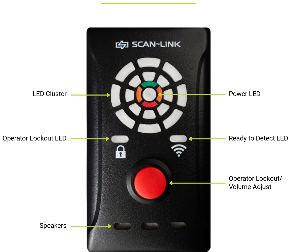
Figure 4: SCAN~LINK Display Unit Diagram
