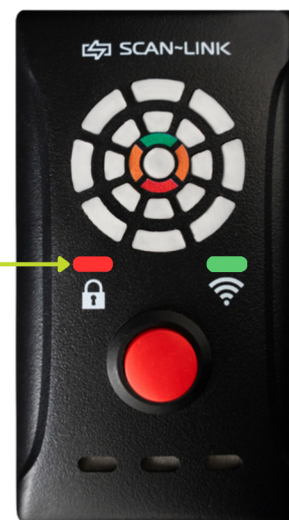
Figure 6: 3.0 Display Unit with Operator Lockout engaged
