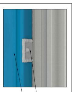
TOOLED SEALANT OVER SCREWHEAD
