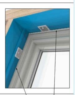
TOOLED SEALANT AT PERIMETER
