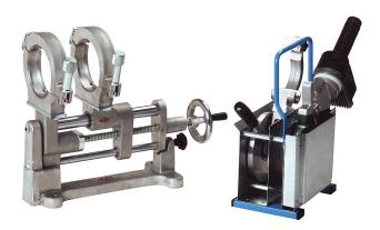
For field and bench fabrication using butt fusion on PE, PP and PVDF pipes and fittings. This machine is detachable from the base unit, allowing on site welding in very small and confined spaces, such as above ceilings and below raised floors. Standard power requirement is 110v. Machine options include Ratchet or Electric Planers, IPS or Metric Reducer Inserts, and a choice of power requirements (110v or 230v).
