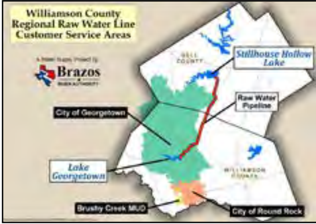
Brazos water pipeline- Courtesy Graphic A pipeline moves water from Stillhouse Hollow Reservoir to Lake Georgetown, and the flow of water south could increase over the next several years to keep up with water demands.
