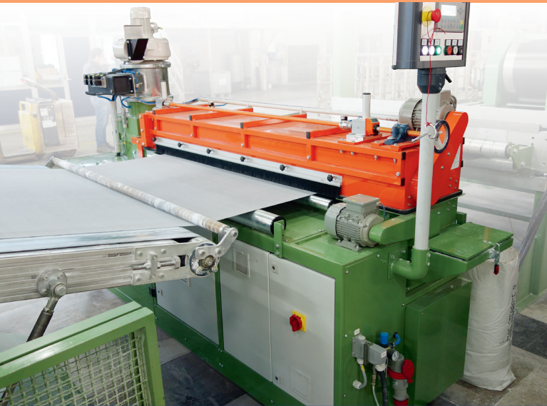
PM 1500 RB For calendered products of up to 3000 mm
