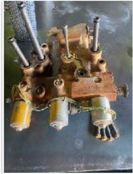
Selector valve removed prior to disassembly.
