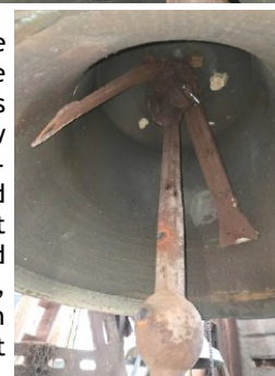
Pictures of some of the "inner workings" of our church bells. You can see that these parts, original with the installation of the bells in 1890, have worn considerably over the years.
