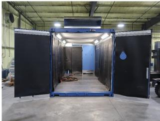
the opposite end of the booth. Ventilation rate is 100 feet per minute. Our cross flow high entry inlet is designed for optimized air and material distribution.
