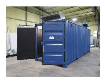
Clean air is introduced into the booth through air inlet plenum field installed on top of the container at the front of the enclosure and is exhausted through blower exhaust at the rear of the booth. Air is pulled horizontally from the front of the booth through the working depth at an average velocity of 100 fpm. The intake and exhaust filter layout are designed for even air velocity throughout the working area of the booth.
