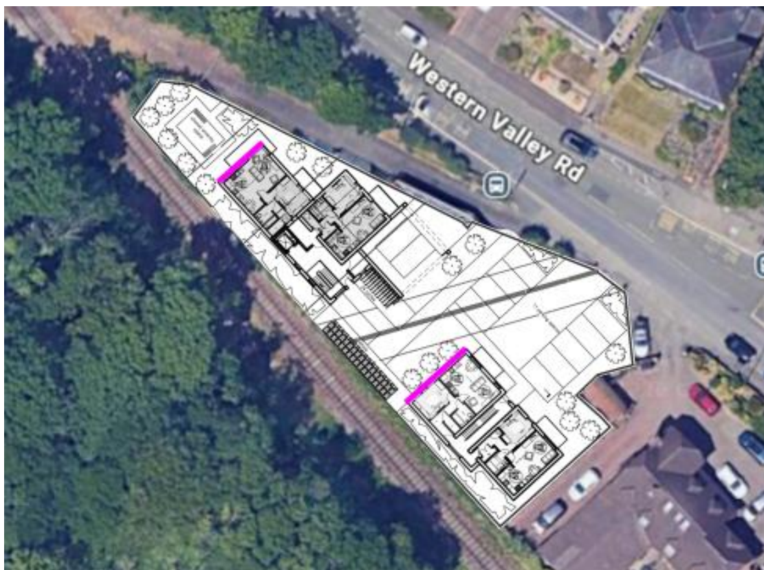
Figure 5.1 – Façades Requiring Additional Sound Insulation Measures
