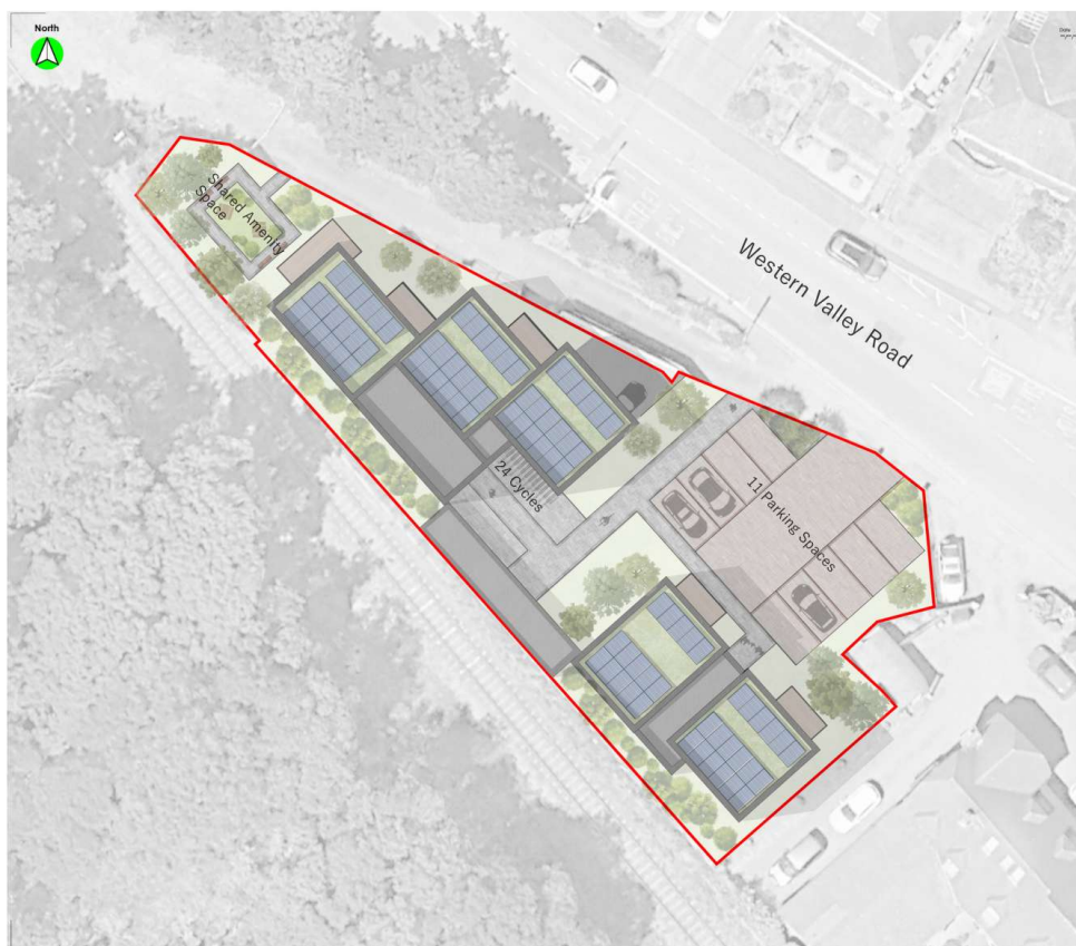
Figure 4: Current proposed site plan, C2J Architects AL(90)10 Revision E. The northern shared garden, two blocks, central parking and cycle provision are shown.
