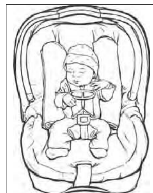
Figure 4. Car safety seat with a small cloth between the crotch strap and infant; chest clip positioned at the center of the chest, even with the infant's armpits; and tightly rolled receiving blankets on both sides of the infant.
