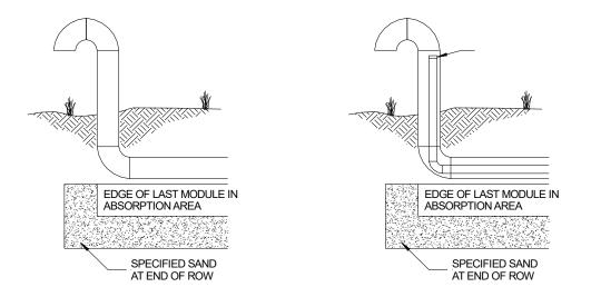
**8.3 VENTILATION PLACEMENT:** In a GSF system, the vent is usually a 4-inch diameter pipe extended to a convenient location behind shrubs, as shown in the figure below. Corrugated pipe may be used. If using corrugated pipe, ensure that the pipe does not have any bends that will allow condensation to pond in the pipe. This may close off the vent line. The pipe must have an invert higher than the system so that it does not drain effluent.
