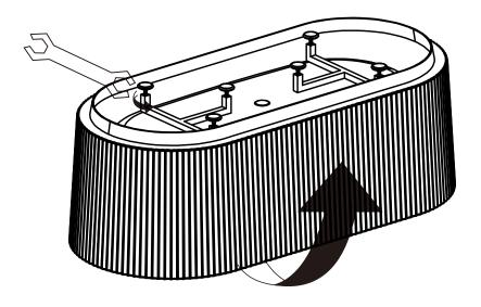
Turn the bath over and temporarily place in what will be final position in the bathroom. Check along the top of the bath using a spirit level and adjust the feel if necessary and lock into place.
