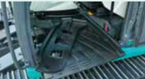
Detachable two-piece floor mat has handles for easy removal. The mat's raised edges trap dirt and grit for easy cleaning.
