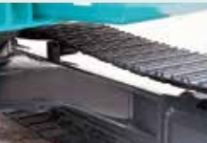
Special crawler frame design makes it easy to clean off mud.
