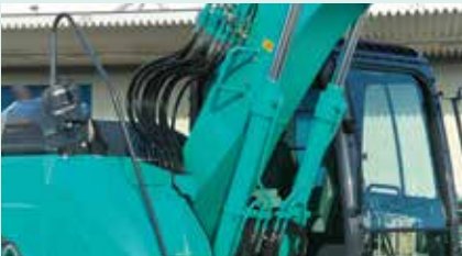
Handhold The handrail is placed on the boom side. In addition, the distance between the current handrails was increased to allow easier access to the maintenance port on the upper arm.
