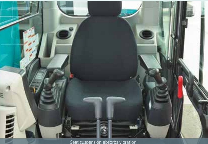
Seat suspension absorbs vibration
