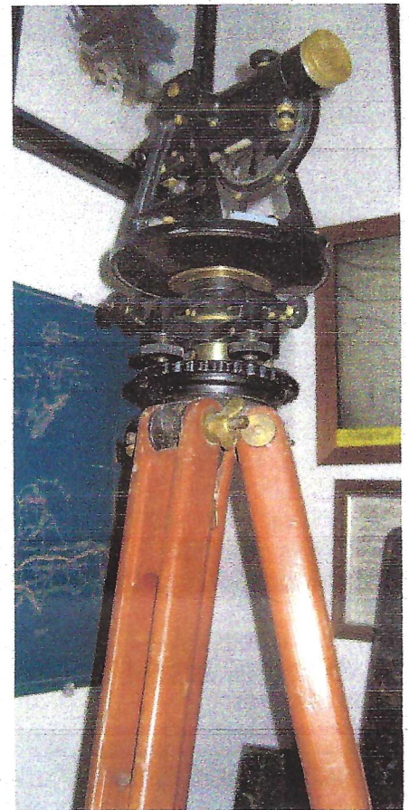
John Papcun donated the pictured surveyor's transit in its wood carrying case with tools. John and his father both served as Ottawa County Engineers, surveying farms and roads with the transit.
