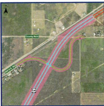
Shifted the side road connecting County Road 6 to Old U.S. 54 and added a right turn taper from W.B. U.S. 54 to turn west onto County Road 6.
