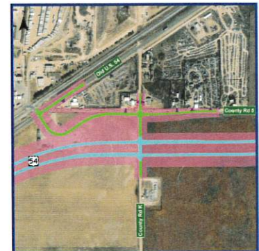
Extended and shifted County Rd 5 and extended work along Old U.S. 54
