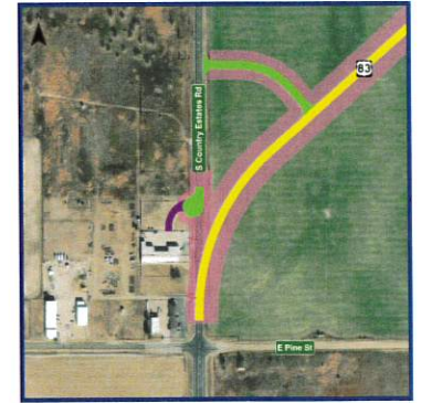
Extended U.S. 83 improvements south to Pine Street, shifted the connecting side road to the south
