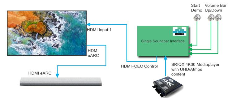
In rest mode the TV is displaying The idle loopvideo when the demo button is pressed the TV displays the demo content while the soundbar is playing back the audio.
