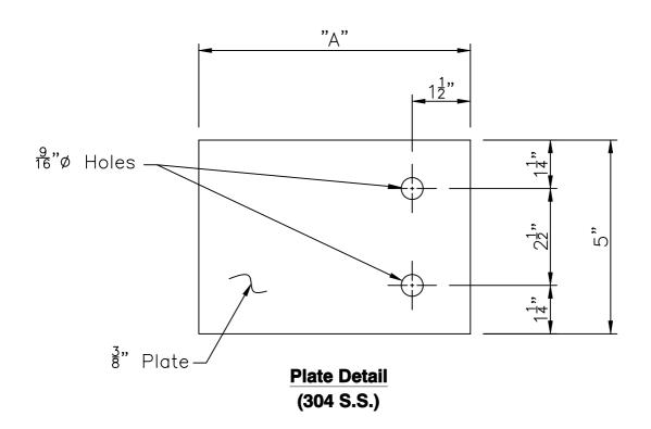
In this application position the edge of the AWS at the center of the hot face material. Therefore dimension "A" will vary to accomodate specific lining thicknesses. The 7" dimension from the edge of the AWS to the holes in the SW3 remains constant.
