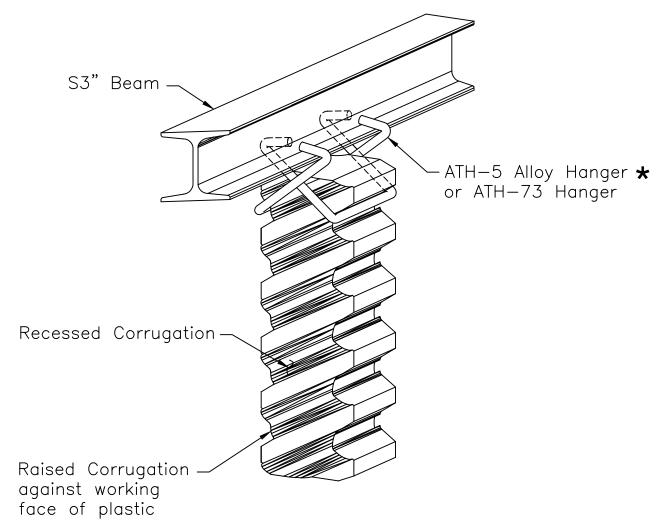
**Arch/Roof Anchor Arrangement**
