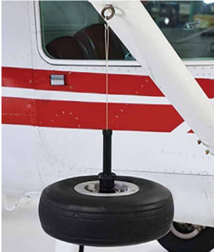
Example of Static Wheel Balancing
