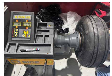
Example of Dynamic Wheel Balancing
