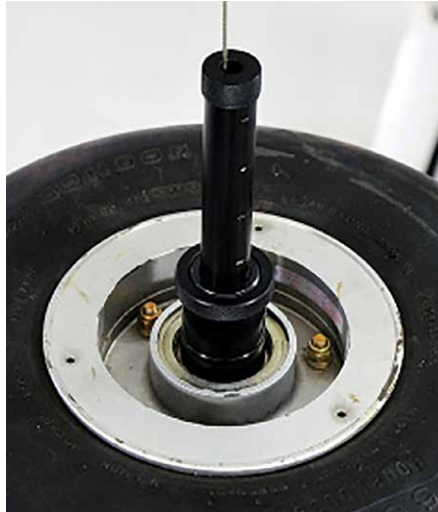
Example of Static Wheel Balancing
