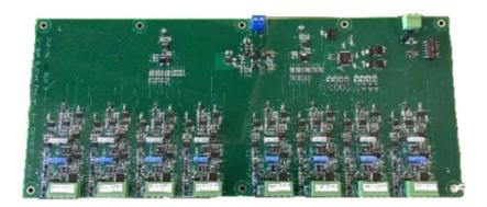
The CVM-XC is a robust, full-range electrical measurement solution engineered for precision, scalability, and reliability. With 8 fully independent channels, it delivers accurate current and voltage measurement for up to 8 Devices Under Test (DUTs) simultaneously—ideal for advanced test stands and engineering validation environments.
