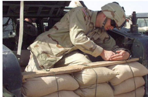
US soldier utilizing sandbags as improvised armor against IEDs.
