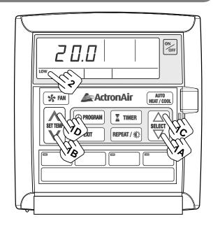
Default Upper and Lower Limits = Upper (30°C), Lower (16°C) It is recommended not to adjust the upper and lower limits outside the defaults above. Doing so, may cause damage to your system and void warranty.
