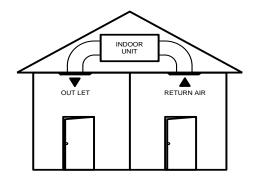
Dust off the outlets and return air, use a household duster. Do this regularly to prevent any build up of dust or dirt.
