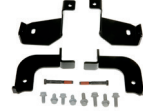
Catcher Adaptor Kit Suits ZTS models - required when fitting a catcher Part # 490-950-C062
