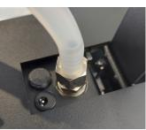
Connect the hose to the burner by inserting the studs.
