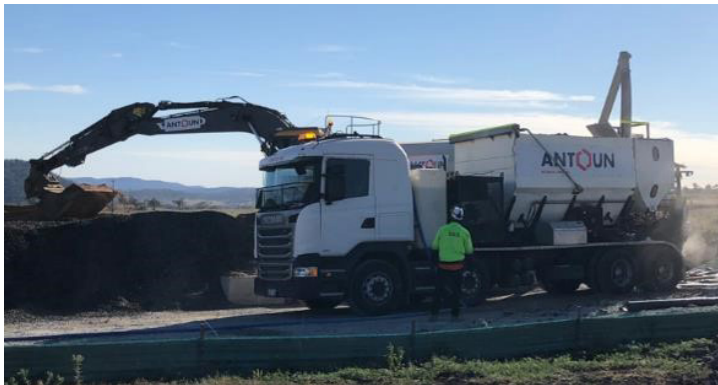
Volumetric Mixer used as a fixed batch plant – 20 cubic metre per hour capacity
