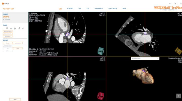
The colors of the lines and borders are corresponding with the orthogonal intersection planes of the MPR. In the example left side, the two red lines in the upper viewport are representing the intersection with the view in the lower left viewport.
