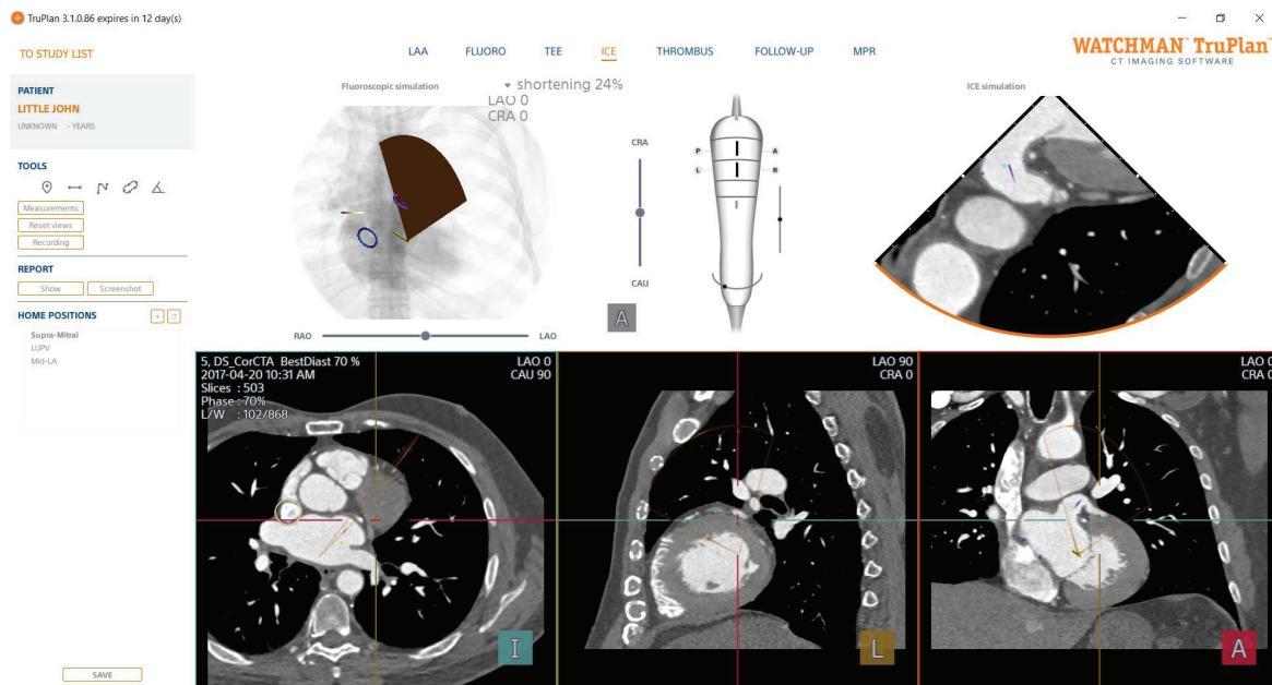
The home positions are listed on the left side and can be selected by clicking on them. Then the probe can be controlled using the virtual probe handle.
