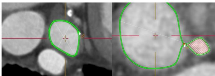
The landing zone contour can be adjusted by dragging the control points that appear when hovering over the green line with the mouse.
