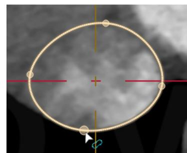
It is possible to resize the contour by dragging the control points that become visible when hovering the mouse over the annotation. It is also possible to insert additional control points.
