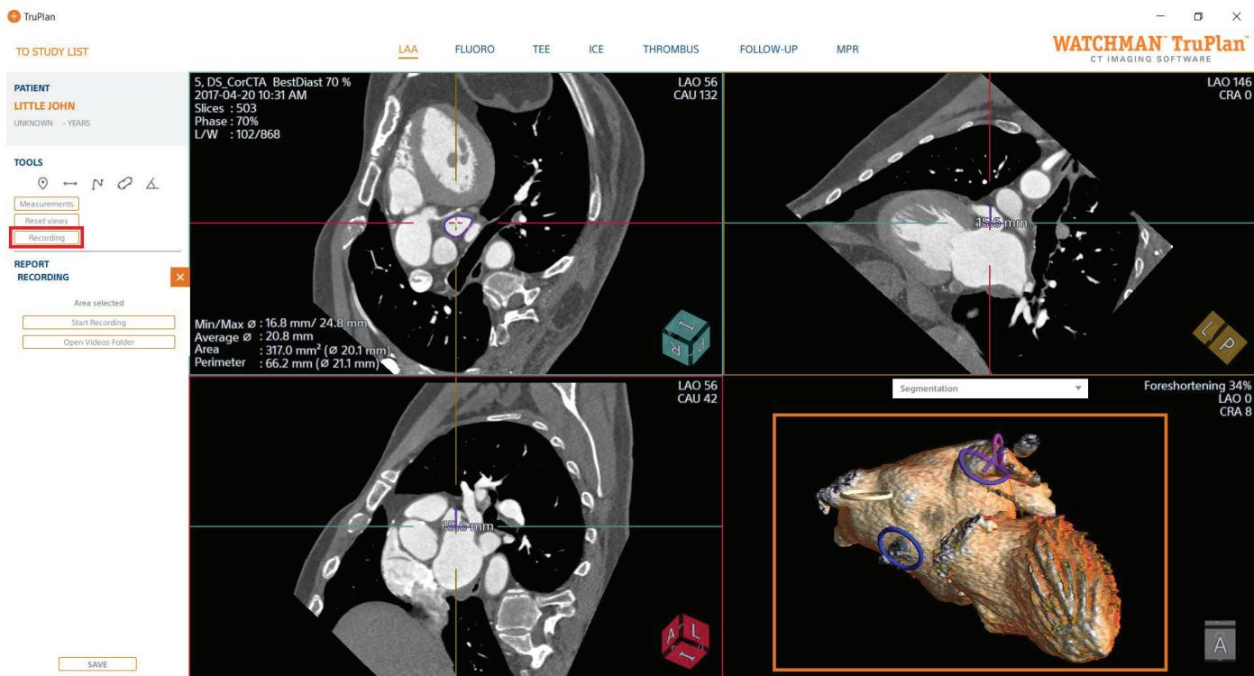
Press the Recording button, then define the area that needs to be recorded: left click on the top left corner of the target area keep the mouse button down and drag the area of interest.
