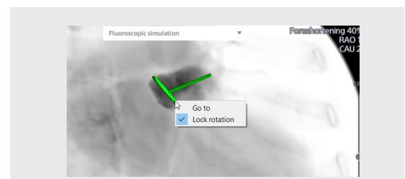
When the Lock rotation option is enabled, the rotation in the fluoro view will be limited to the angles that will show the landing zone in a perpendicular way.
