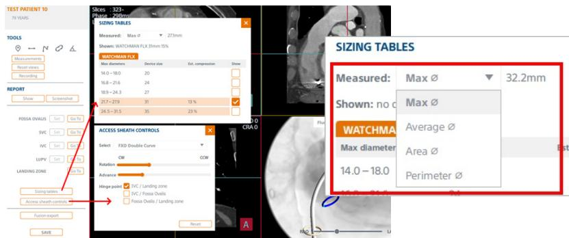
Open the Sizing tables dialog for the available devices, select the desired device. (Support for the WATCHMAN 2.5 can be enabled via the configuration menu.)
