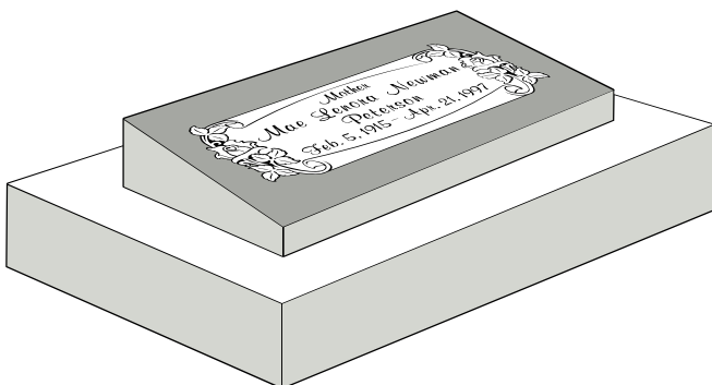
STONE SET IN CONCRETE ON SLOPE
