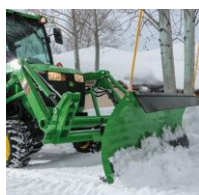
Front Blade Clear snow and move dirt or gravel. Angle right or left to make the job easier. Snow pushes also available.
