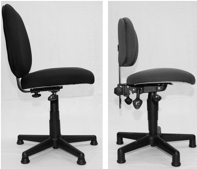
Figure 3. The task chair with a flat seat pan is on the left, and the chair with a curved seat pan is on the right. Both chairs are adjustable in height. The chairs have no castors so that they do not move during sewing.
