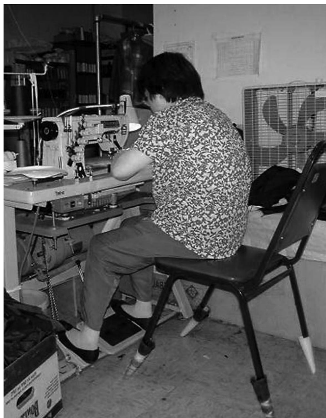
Figure 1. Typical posture of sewing operator with a conventional chair. Note flexed postures of thoracic and cervical spine and abduction of shoulder. Note also that the operator increased the height of the chair with paper cones.
