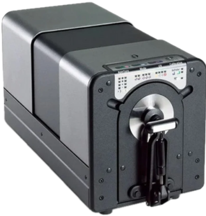
Color Spectrophotometer used during ASTM D2244 to evaluate and standardize color measurements of material samples before and after accelerated UV exposure testing.
