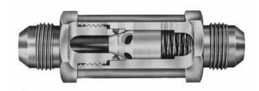
These spring-operated poppet valves, with optional relief settings, allow free flow in only one direction and prevent backflow - sometimes referred to as "backflow preventor", "flow stop", or "non-return" valve. They are also used for relief and bypass functions.
