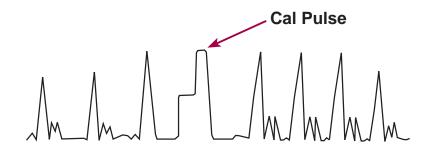
Two levels of calibration pulses are provided. While Cal is active, calibration tones synchronised to the calibration pulses are superimposed on the audio signal.
