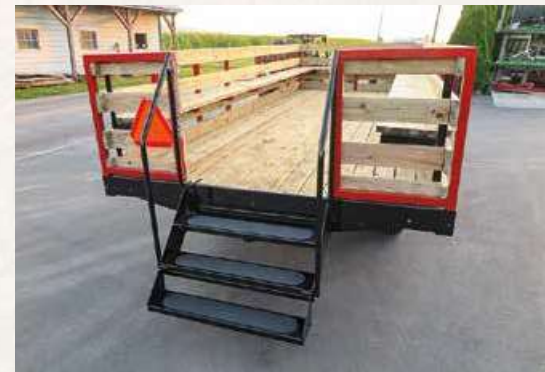
Rear step folds down for easy loading.
