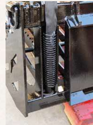
90 degree quick couplers and a tension spring keep hoses away from pinch points.
