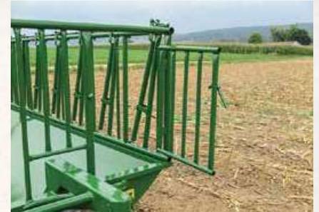
Front gate allows easy access to inside of feeders
