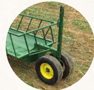
Tongue can be fastened in the upright position
