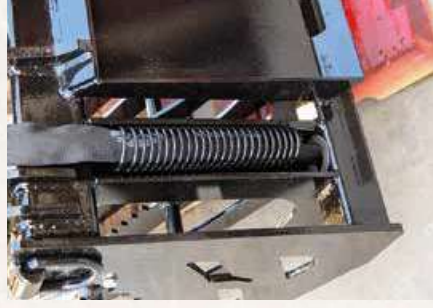
90 degree quick couplers and a tension spring keep hoses away from pinch points.
