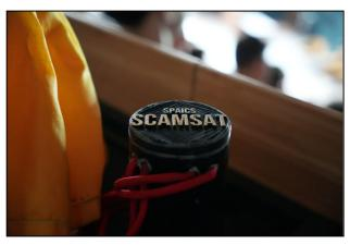
These two disks are used later on and placed within the CanSat. The middle disk is screwed in from outside with a washel and screw using a high power drill. The top cap stays firm during descent as tested due to the perfect fit pressure, and the lock from the parachute. This cap allows easy access to the inside as well.
