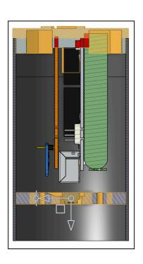
The two images above show the combination of disks, image on the left shows the way that these two disks will be placed together onto the PVC. The PVC in the above image does not show any holes for parachute or screws for easy representation. The image on the right shows a cross/sectional view of the can with primary electronics inside. Once the disks are attached. The electronics can be placed inside the can:
