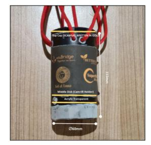
using a Ø60mm PVC Pipe to ensure a strong body. There will be many small holes in the middle cap for the APC to transmit data well hence it will not protrude outwards the given dimensions. The parachute will be made of soft material and will fold within the given extra 4.5cm. Hence all CanSat dimension requirements will be met.
