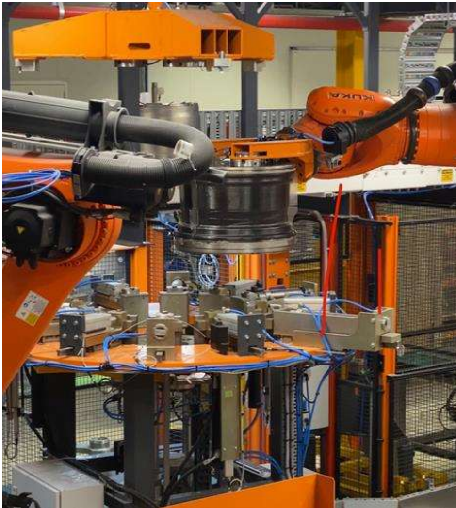
Figure 8 Carbon Revolution Mega-line demoulding station: the mould tools, preserve precise part geometries upon demould.
