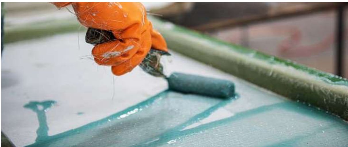
Figure 14 Open mould, hand lay-up process: Resin is applied manually to each layer using a brush or roller, followed by consolidation to eliminate air pockets and achieve uniform resin distribution. The part is then left to cure at ambient temperature or under controlled heat.
