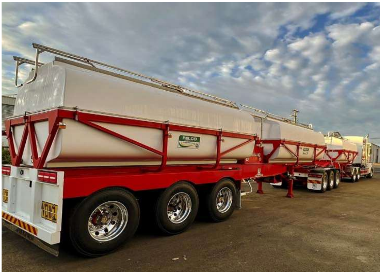
Figure 18 Felco's truck and semi-trailer mounted bulk liquid haulage tankers - ranging between 2000 to 20,500 litres capacity - are fully engineered and tested, and then handcrafted by the Felco team of advanced composite technicians in Toowoomba. Photo by Rod Monti.
