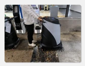
3. Use the key to power off the robot and wait for the screen off.
