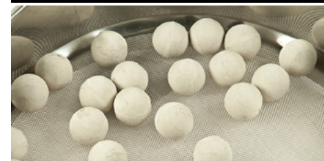
1. Cleaning brushes for sieves. 2. Food balls used to open the mesh of sieve.
