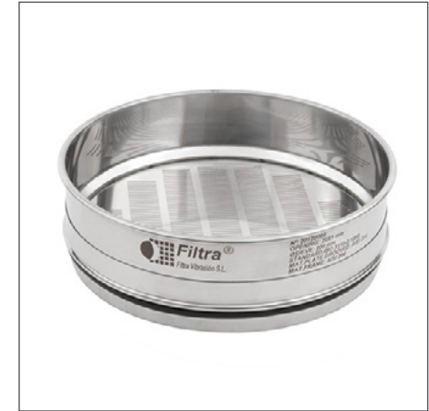
Stainless steel sieve with oval perforated plate (for cereals, ISO 5223).
